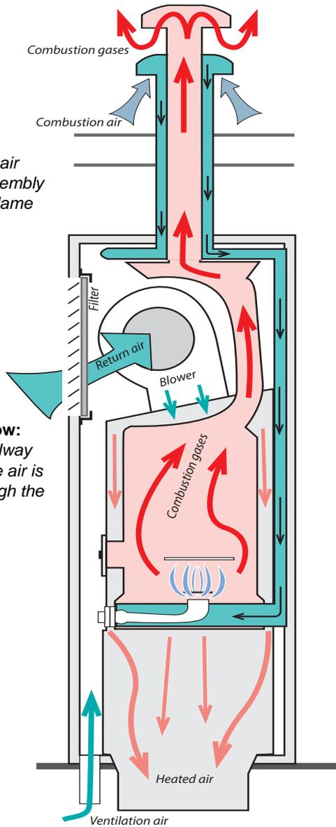
**Mobile-home furnace airflow:** *Return air flows from the hallway through the furnace grill. The air is heated and distributed through the*
