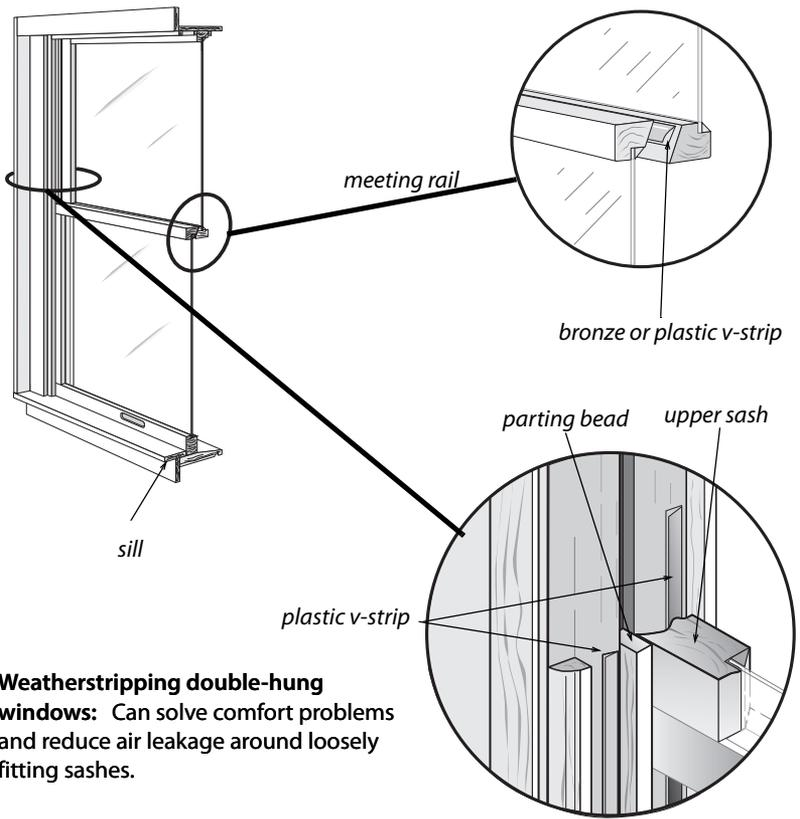
**Weatherstripping double-hung windows:** Can solve comfort problems and reduce air leakage around loosely fitting sashes.
