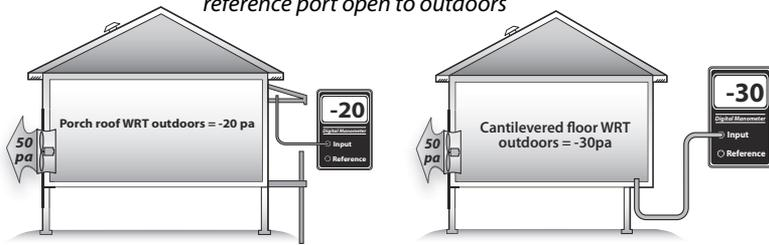
**Porch roof test:** If the porch roof were outdoors, the manometer would read near 0 pascals. We hope that the porch roof is outdoors because it is outside the insulation. We find, however, that it is partially indoors, indicating that it may harbor significant air leaks through the thermal boundary.
