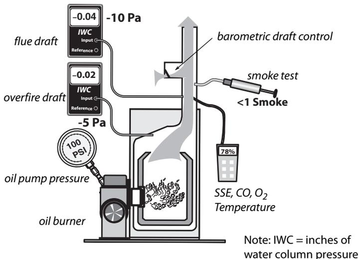
**Measuring oil-burner performance:** Measuring oil-burning performance requires, a manometer, flue-gas analyzer, smoke tester, and pressure gauge.
