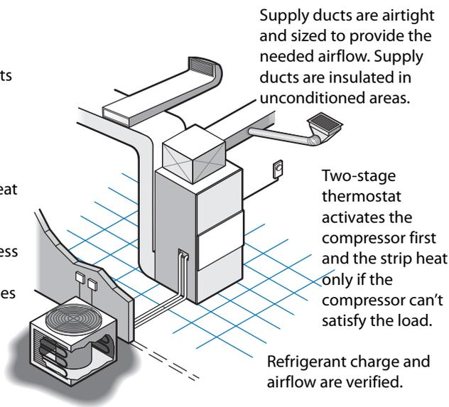
Coil is cleaned every year. Weeds, grass and shrubs shouldn't grow within 3 feet. Verify that no airflow restrictions exist above the outdoor unit.
