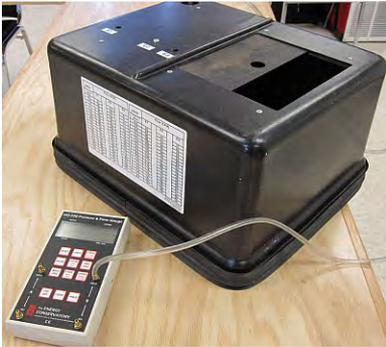
**Measuring fan airflow:** Use an exhaust-fan flow meter or a flow hood to verify the airflows through local exhaust fans and whole-building ventilation fans.
