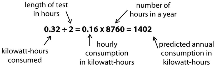
**Refrigerator consumption example:** In this example, a 2-hour measurement was performed. During this time, the appliance consumed 0.32 kilowatt-hours of electricity, or 0.16 kilowatt-hours per hour. The annual total of 1402 kilowatt-hours, calculated above, is well beyond the 450 kilowatt-hours per year consumed by today's most efficient refrigerators.
