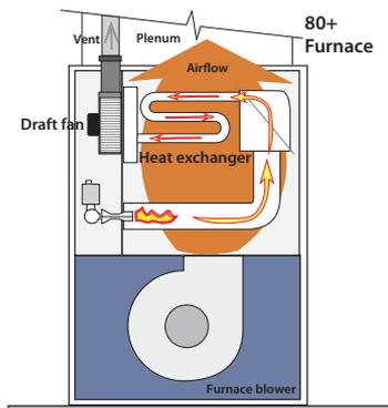
**80+ Gas furnace:** An 80+ furnace has a restrictive heat exchanger and draft fan, but has no draft diverter and no standing pilot light.
