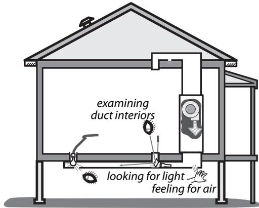
1. Use the air handler blower to pressurize supply ducts. Closing the dampers on supply registers temporarily or partially blocking the register with pieces of carpet, magazines, or any object that won't be blown off by the register's airflow increases the duct pressure and make duct leaks easier to find. Dampening your hand makes your hand more sensitive to airflow, helping you to find duct air leaks.
