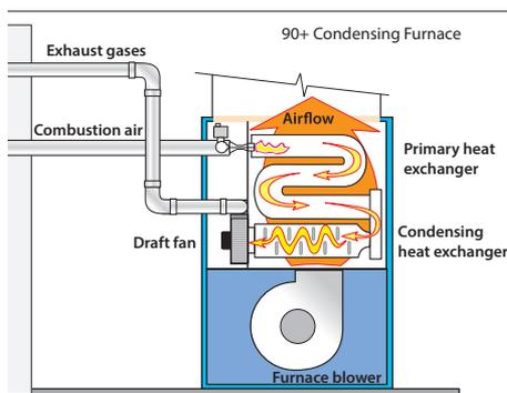
**90+ Gas furnace:** A 90+ furnace has a condensing heat exchanger and a stronger draft fan for pulling combustion gases through its more restrictive heat exchanger and establishing a strong positive draft.
