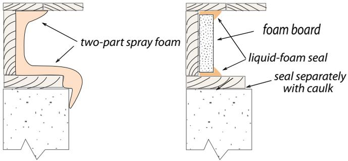
**Foam-insulated rim joists:** Installing foam insulation is the best way to insulate and air seal the rim joist.
