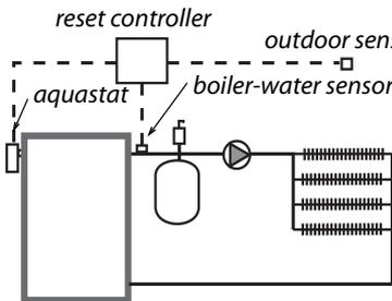
**Reset controller:** This control adjusts circulating-water temperature depending on the outdoor temperature.
