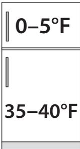
**Refrigerator clean and tune:** Clean coils and check temperatures. Adjust temperatures that are out of range.
