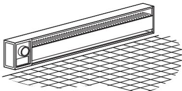
**Electric baseboard:** Electric baseboard is more efficient than an electric furnace and sometimes even outperforms a central heat pump because it is easily zone-able. The energy bill is determined by the habits of the occupants and the energy efficiency of the building.
