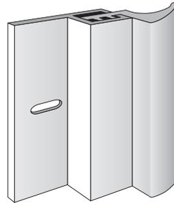
*This Q-Lon weatherstrip installs on an existing door stop.*
