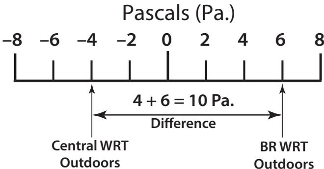
**Measuring unbalanced airflow:** The distance on a number line represents the difference in pressure between the central zone and the bedroom.
