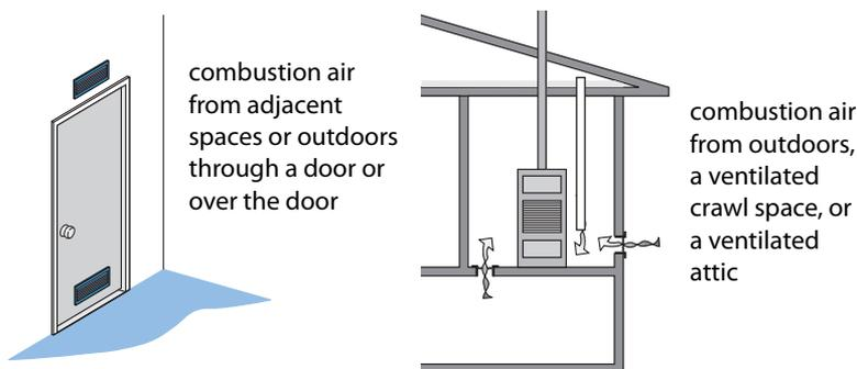
**Combustion air options:** Combustion air can be supplied from adjacent indoor spaces or from outdoors. High vents may occasionally compete with chimney draft for available air. Beware of drawing combustion air from wet crawl spaces. Pick your outdoor combustion-air location carefully to avoid pressurizing or depressurizing the CAZ.
