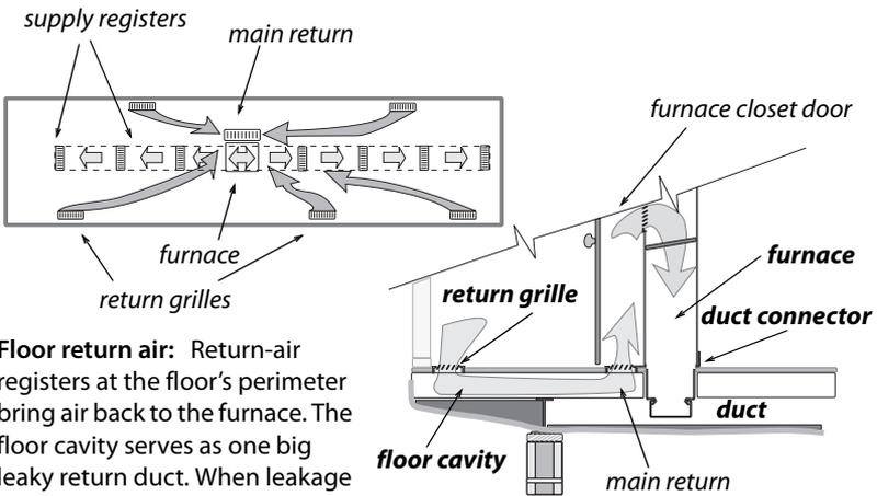
**Floor return air:** Return-air registers at the floor's perimeter bring air back to the furnace. The floor cavity serves as one big leaky return duct. When leakage is serious, the floor return system should be eliminated.
