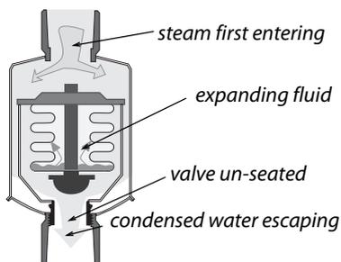
**Steam traps:** Steam enters the steam trap heating its element and expanding the fluid inside. The expanded element plugs the steam's escape with a valve.
