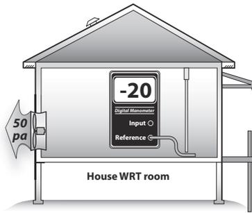
**Bedroom test:** This bedroom pressure difference may be caused by its leaky exterior walls or tight interior walls, separating it from the main body of the home. This test can determine whether or not a confined combustion zone is connected to other rooms.
