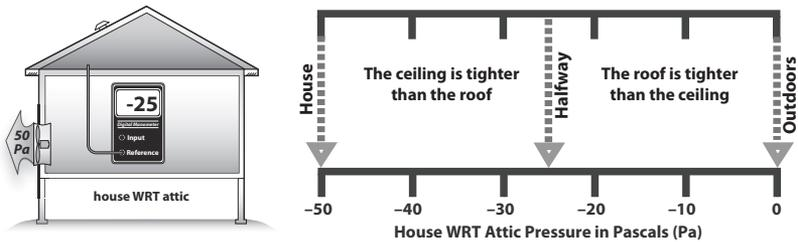
**Building-to-attic pressure:** This test allows the tester to evaluate the attic's two possible air barriers—the ceiling and the roof. The diagram shows how to determine which air barrier is tighter.
