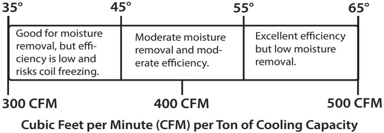
**Coil temperature and airflow:** The ideal airflow and coil temperature vary by the average relative humidity of a local climate.
