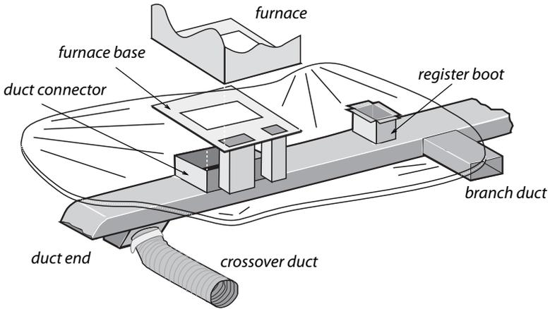
**Mobile-home ducts:** Mobile-home ducts leak at their ends and joints — especially at the joints beneath the furnace. The furnace base attaches the furnace to the duct connector. Leaks occur where the duct connector meets the main duct and where it meets the furnace. Branch ducts are rare, but easy to find, because their supply register isn't in line with the others. Crossover ducts are found only in double-wide and triple-wide homes.
