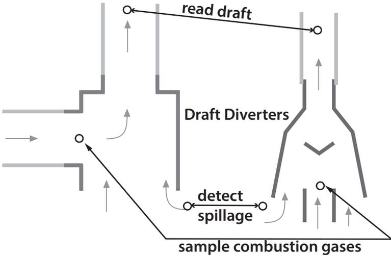
**Testing locations:** This illustration shows two draft diverters and the locations (circles) for draft testing, spillage detection, and sampling of combustion gases.
