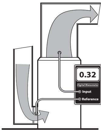
**Static pressure and temperature rise:** Measure static pressure and temperature rise across the new furnace to verify that the duct system isn't restricted. The correct airflow, specified by the manufacturer, is necessary for high efficiency.
