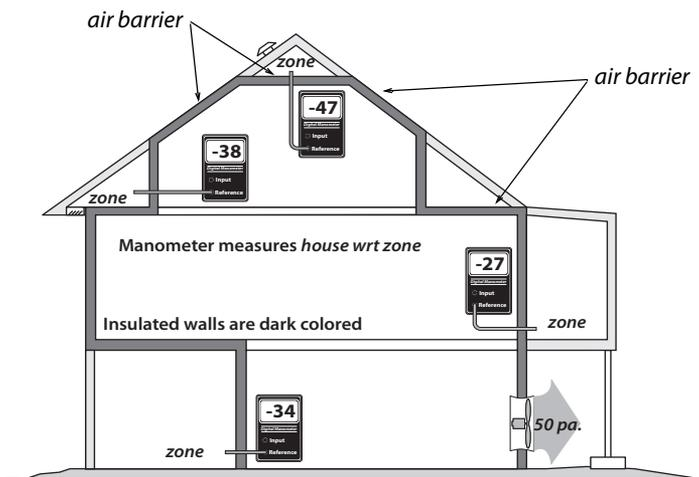
**Pressure-testing building zones:** Measuring the pressure difference across the assumed thermal boundary (*house wrt zone*) tells you whether the air barrier and insulation are aligned. If the manometer reads close to  $-50$  pascals, the air barrier and insulation are aligned and the tested zones are well-connected to outdoors.
