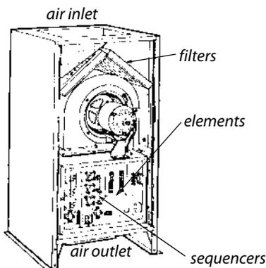
**Electric furnace:** A squirrel-cage blower blows air over 2 to 6 electric resistance coils and down into the plenum below the floor.
