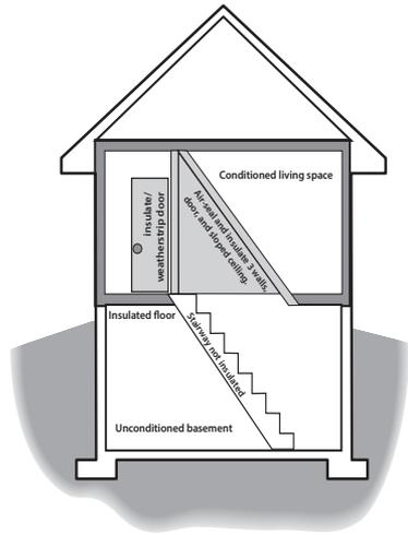
**Stairways at the thermal boundary:** The stairway may be within the thermal boundary or outside it. Only walls, ceilings, doors, and hatches at the thermal boundary require thorough air sealing. The door as shown is open.
