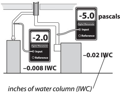
**Measuring draft:** Measure chimney draft *downstream* of the draft diverter.
