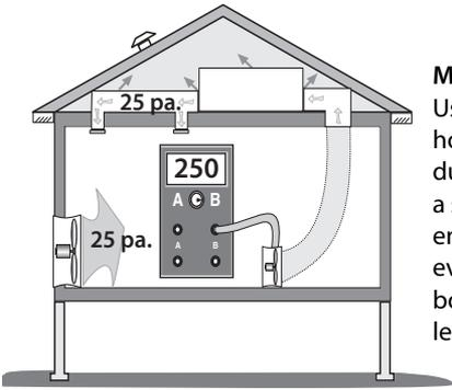
**Measuring duct leakage to outdoors:**
