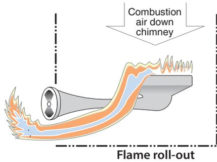
Take all necessary steps to reduce CAZ depressurization and minimize combustion spillage, based on your tests.
