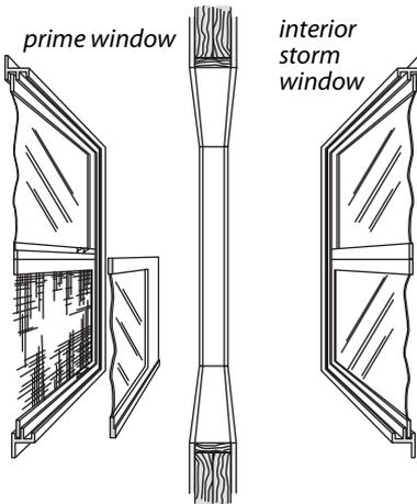
**Mobile-home double window:** In mobile homes, the prime window is installed over the siding outdoors, and the storm window is installed indoors.
