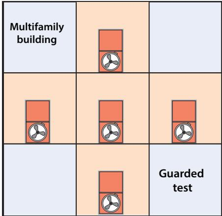
**Guarded test:** Attempts to measure the leakage to outdoors of a single dwelling unit. One blower door measures the units air leakage while other blower doors pressurize adjacent units to the same negative or positive pressure.
