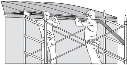
**Roof-edge blowing:** Use a rigid fill tube to blow insulation through the roof edge. This avoids making holes in the roof itself, though this process requires much care in refastening the roof edge.
