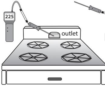
**CO from range and oven:** Measure CO at oven in undiluted flue gases. Measure ambient CO in the area of the range, but not directly above the burners or oven vent.
