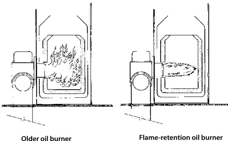
**Flame-retention burner:** The flame of a flame-retention burner is hotter and more compact than the older burner.
