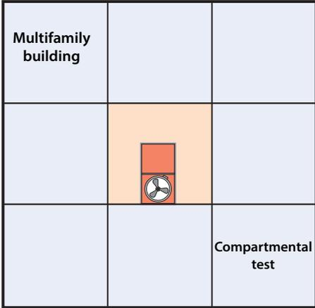
**Compartmental test:** A single blower door pressurizes a single dwelling unit. Identifies features of the unit that leak air to the outdoors and to surrounding units.
