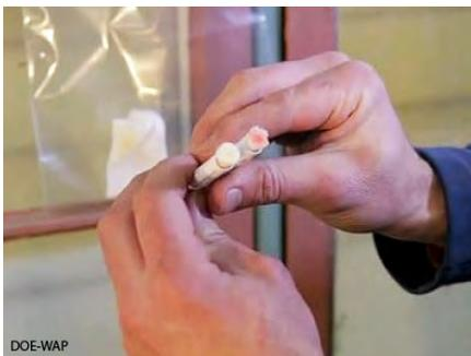
Red means lead-positive and white means lead-negative.
