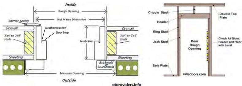
**Door anatomy:** The door and its frame fit into a rough opening. The door jamb matches the wall thickness and attaches to casing on the interior and exterior of the wall.
