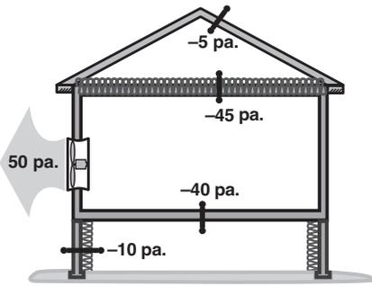
**Pressure measurements and air-barrier location:** The air barrier and insulation are aligned at the ceiling. The crawl-space pressure measurements show that the floor is the air barrier and the insulation is misaligned — installed at the foundation wall. We could decide to close the crawl space vents and air seal the crawl space. Then the insulation would be aligned with the air barrier.
