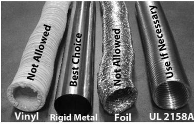
**Dryer vent types:** Clothes dryer energy-efficiency depends on the type of vent material and the equivalent length of the vent.
