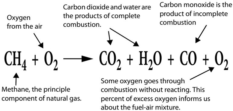
Modern combustion analyzers measure  $\text{O}_2$ ,  $\text{CO}$ , and flue-gas temperature. Some models also measure draft. Combustion analyzers also calculate combustion efficiency or steady-state efficiency (SSE), which are synonymous.
