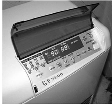
**Space heater controls:** Many modern energy-efficient space heaters have programmable thermostats as a standard feature.
