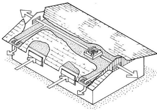
**Whole-house fan circulation:** the whole-house fan sucks air out of the house and exhausts it into the attic or through a gable wall. Cooler air enters the windows as make-up air for the fan.
