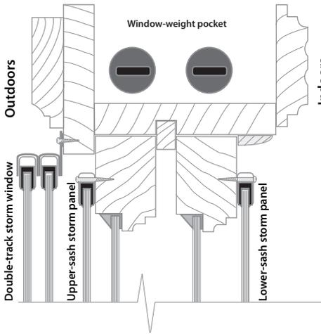
**Optimized double-hung window:** An exterior aluminum storm window plus storm window panels on the window sashes create triple glazing in this double-hung window.
