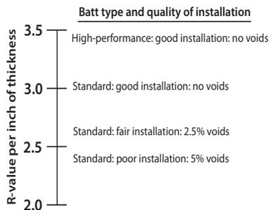
Installers must cut and fit batts very carefully. Batt achieves its advertised R-value only when they are touching all six sides of the cavity it inhabits.
