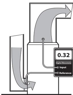
**Total external static pressure (TESP):** The positive and negative pressures created by the resistance of the supply and return ducts produces TESP. The measurement shown here simply adds the two static pressures without regard for their signs. As TESP increases, airflow decreases. Numbers shown below are for example only.
