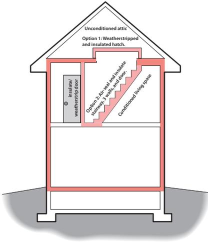
**Stairways at the thermal boundary:** The stairway may be within the thermal boundary or outside it. Only walls, ceilings, doors, and hatches at the thermal boundary require thorough air sealing. The door as shown is open.
