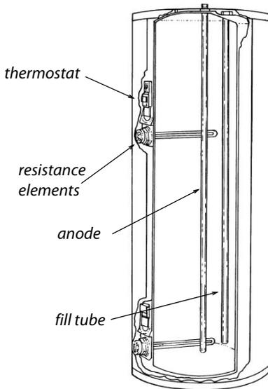
**Standard electric storage water heater:** Electric water heating is more expensive than gas or oil but safer. Electric water heaters should have at least 2 inches of foam insulation.
