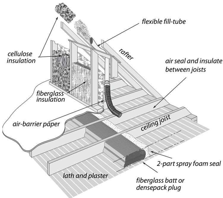
**Finished attic best practices:** Air sealing and insulation combine to dramatically reduce heat transmission and air leakage in homes with finished attics.
